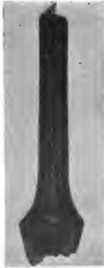
Fig. 30—A dead wood spoke which failed in service
